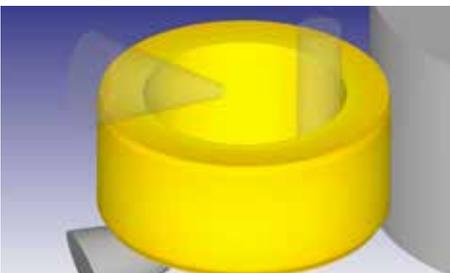
The axial rollers control the height of the ring. The idler roller, or mandrel, applies pressure to the preform by pressing it against the drive roller to decrease wall thickness and height and increase ring diameter until the correct diameter is reached.
