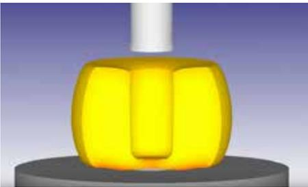
The blank is punched then pierced in the center, using the open die forging process, to create a preform in the shape of a donut.
