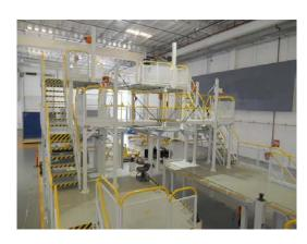
Bombardier Aerospace selected Gonzalez Aerospace to build this 3-level "after-fuse" assembly platform for their new Global 7000 / 8000 aircraft which is being built at their Queretaro Mexico facility
